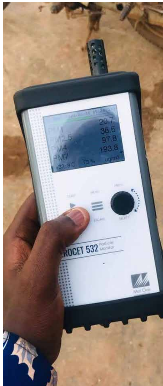
Air Quality Sensor Device used during data collection (HePD, 2024).
